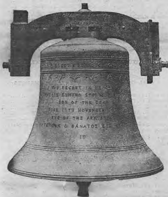
The Recast Tenor (30 cwt.) at ROCHESTER CATHEDRAL.
