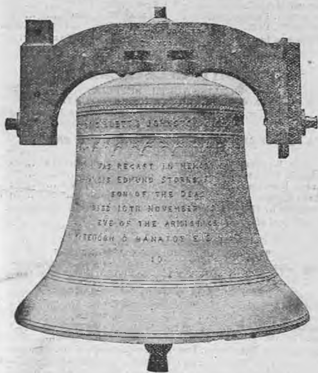
The Recast Tenor (30 cwt.) at ROCHESTER CATHEDRAL. New Ring of Ten opened May 14th, 1921.
