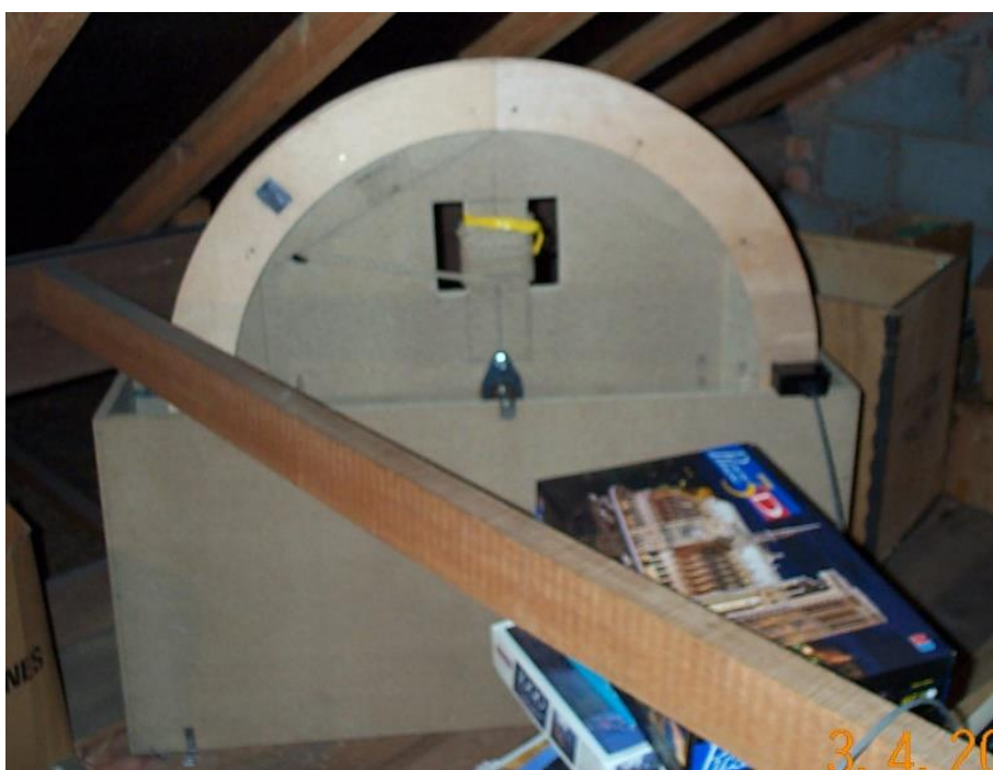
My first dumbbell with homemade sensor mounted in the loft
