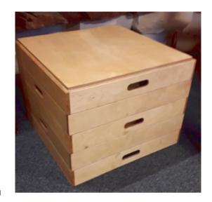
wish. There is about 100mm extra height available from the 8' x 4' sheet after making allowance for cutting wastage. A good use of this might simply be to make three medium height boxes and only four small ones but I chose to have five small boxes as these are the most commonly required.
