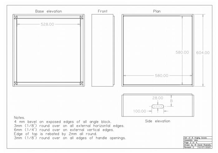
The (long) front and back of each box is the least critical and the cutting list shows 2mm extra length on these so that they can be trimmed after assembly. If the ends are perfectly square it will make assembly easier.
